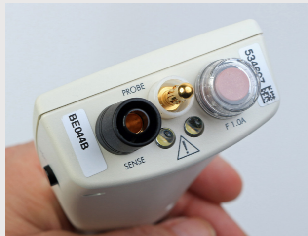
Front with test probe connections, LEDs for illuminating the work area and fuse insert
