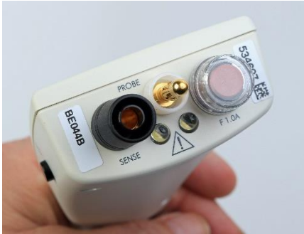
Lateral push-button and 2 light-emitting diodes on the front to light the work area
