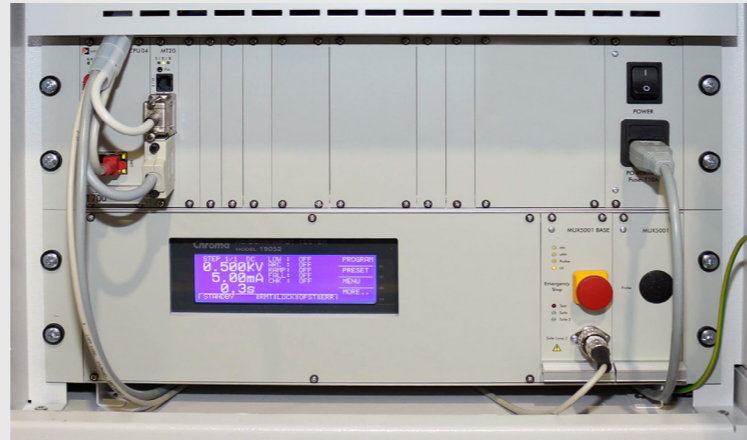
Integrated NT 700-11: CPU and HV generator
