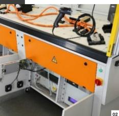
Voltage / compressed air supply and LV and HV test points
