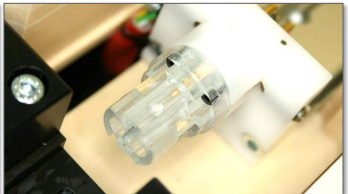
Level with contact carrier and highly precise shadow mask
